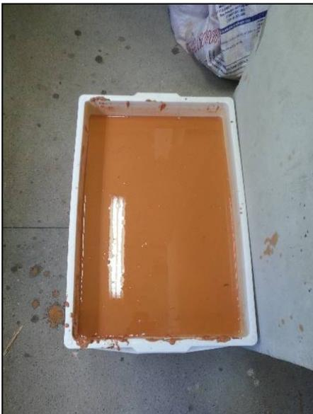
Figura 12. Amostra Solo + H<sub>2</sub>O + NaOH.
