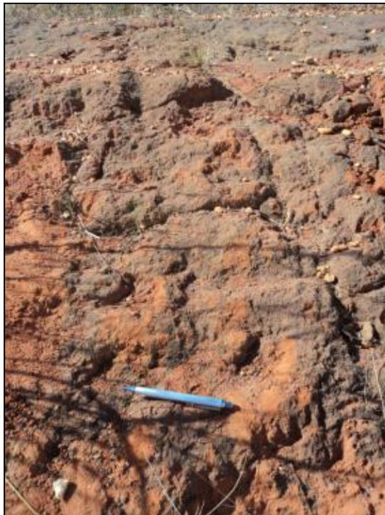
Figura 7. Solo com crosta laterítica. *Figure 7. Soil with lateritic crust.*
