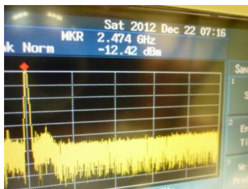
Figure 7.26 - Measured oscillation frequency for \text{OSC}_{\text{N1}}
