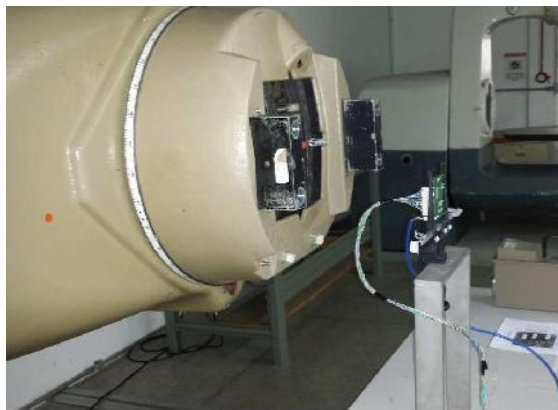
Figure 6.37 - ^{60}\text{Co} source and test circuit inside LRI/IEAv laboratory
