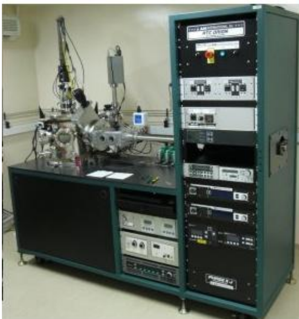
Fig.2. 2 AJA Orion 8 sputtering system used to deposit thin films.
