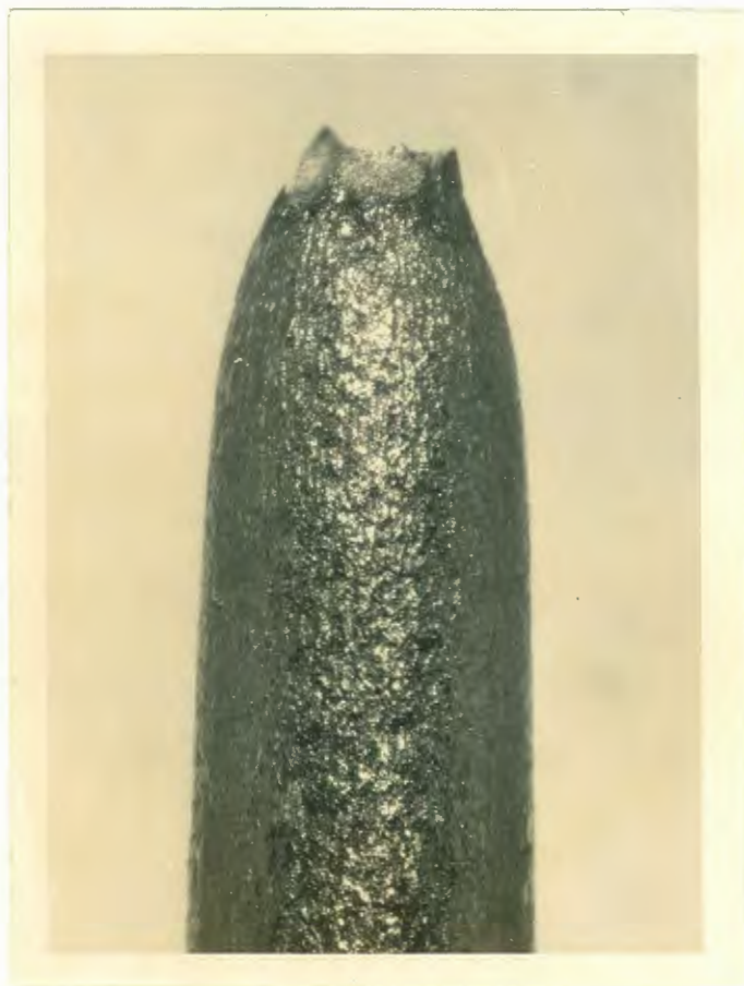
Fig.30. Aspecto geral do CP. 20 x. \text{MgCl}_2 puro, -160 \text{ mV}_H .
