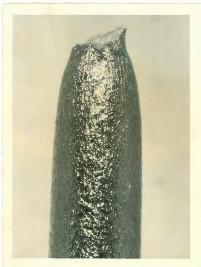
Fig.48. Aspecto geral do CP. 20x. \text{MgCl}_2 + \text{NaNO}_3 . -100 \text{ mV}_H .
