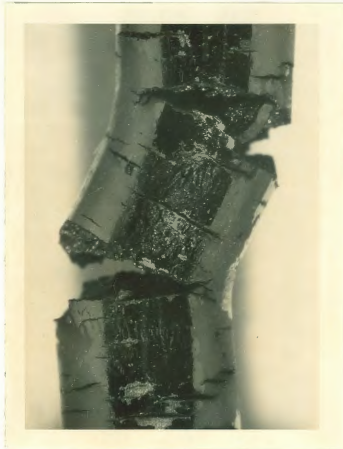
Fig.44. Aspecto geral do CP. 20x. \text{MgCl}_2 + \text{NaNO}_3 . -60\text{mV}_H .
