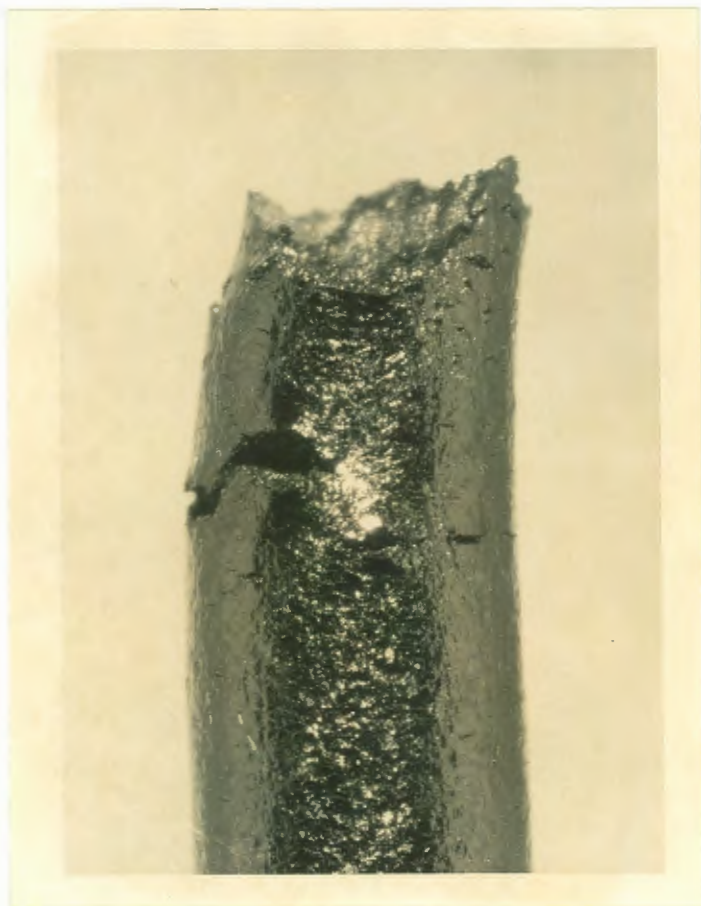
Fig.31a. Aspecto geral do CP. 20x. \text{MgCl}_2 puro, PCL ( -140\text{mV}_H ).
