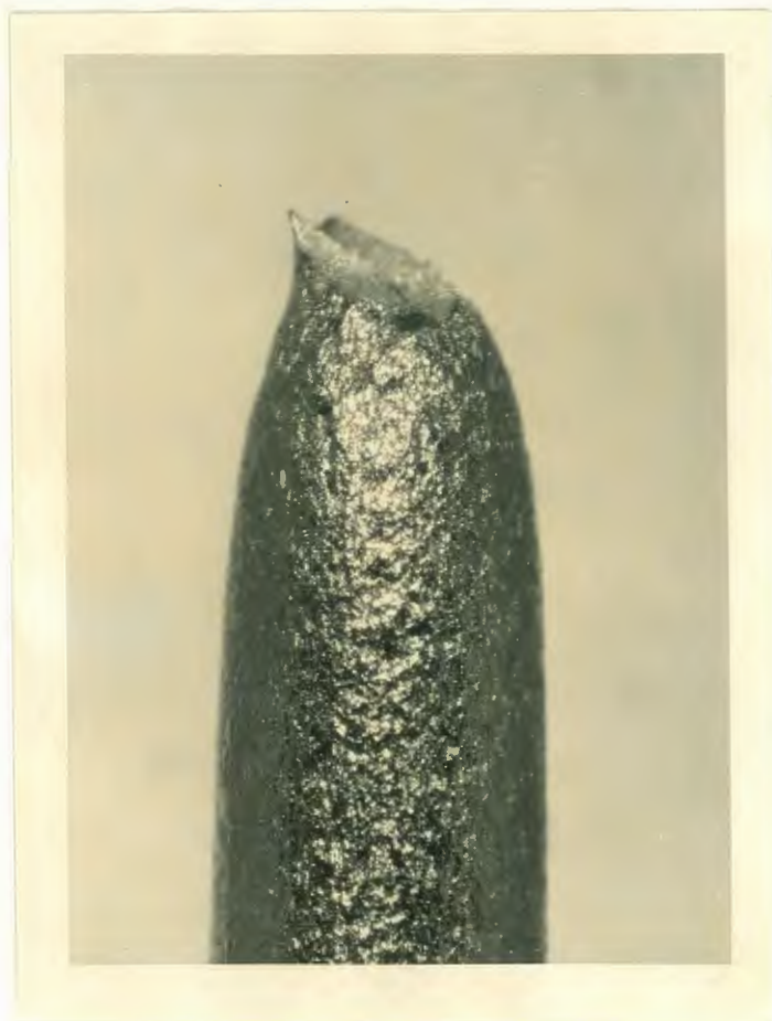
Fig.33. Aspecto geral do CP. 20x. \text{MgCl}_2 + \text{NaNO}_3 . PCL (-145 \text{mV}_H ).
