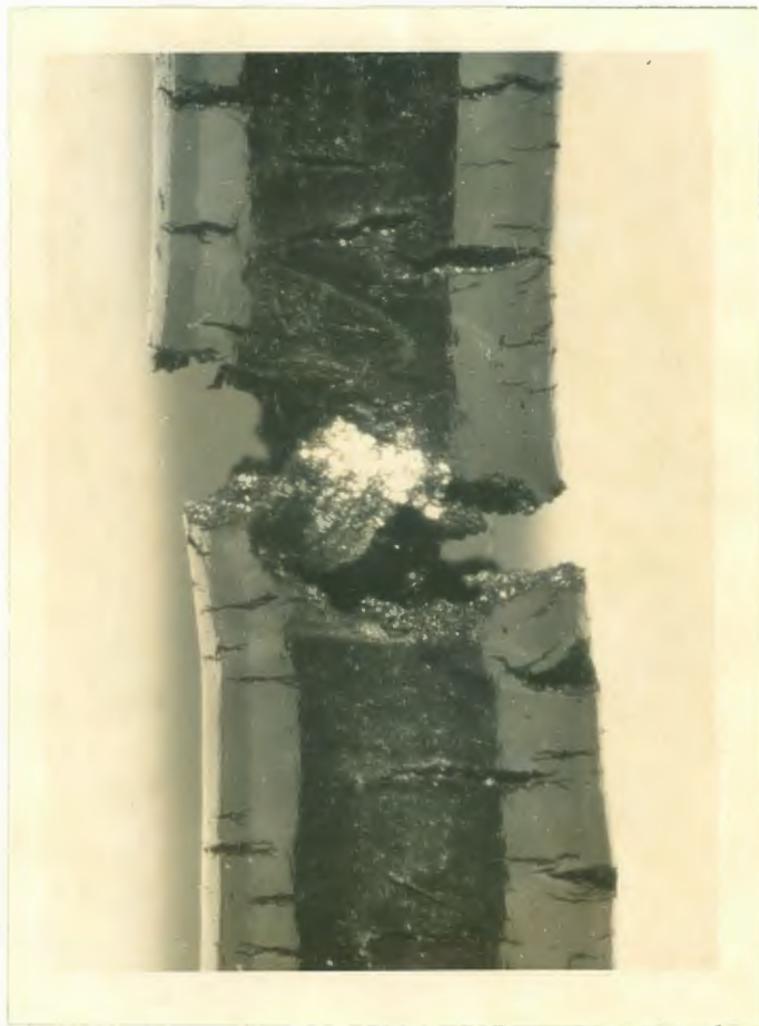
Fig.45. Aspecto geral do Cp. 20x. \text{MgCl}_2 + \text{NaNO}_3 . -70 \text{mV}_H .
