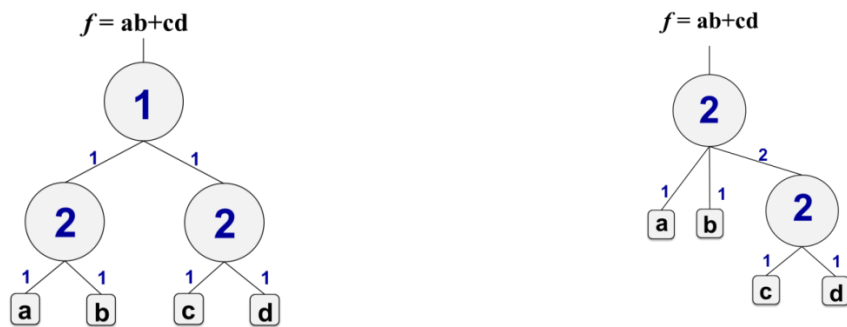
Figure 1.2: Two different TLG networks implementing the function f=ab+cd .
